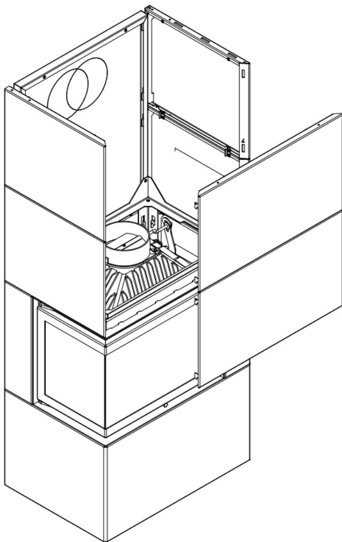
**Step 18:** Install the top frame of the superstructure as shown in the diagram below. Screw the frame to each panel so that the whole structure is adequately stiffened.
