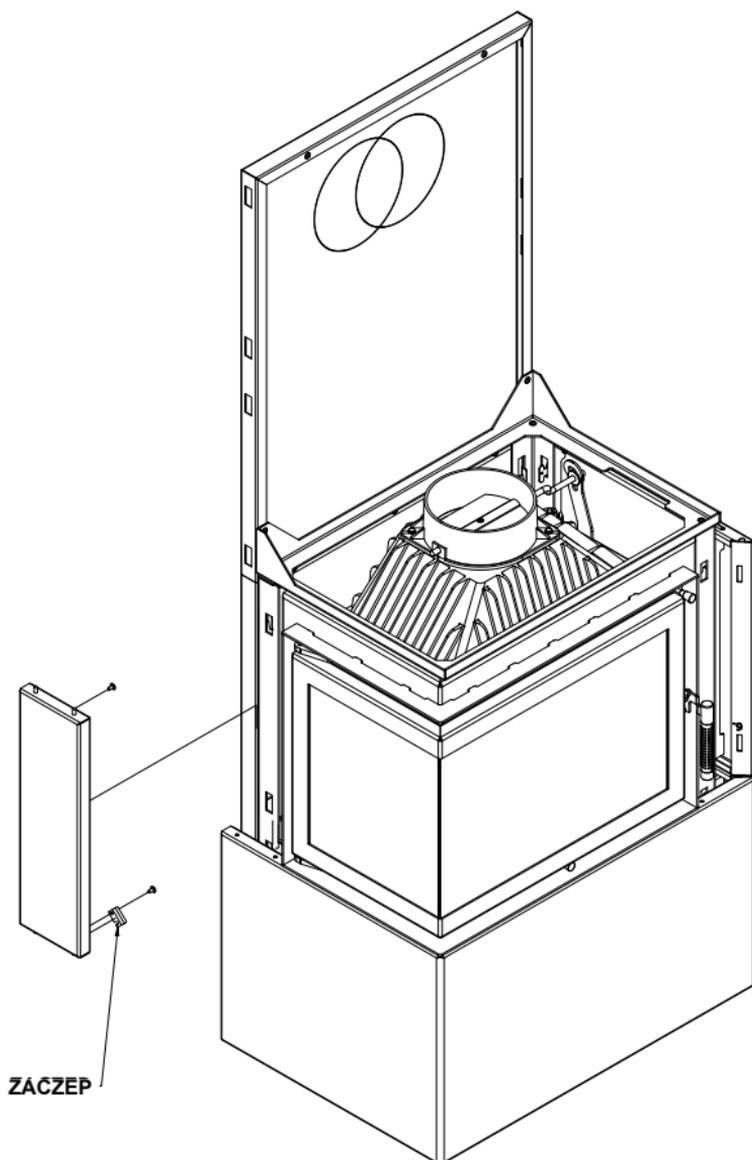
**Step 12:** Prepare the smaller front panel before installing it on the building structure, as shown in the diagram below. Depending on the BSL or BSP version, screw in the appropriate hangers according to the schemes below.
