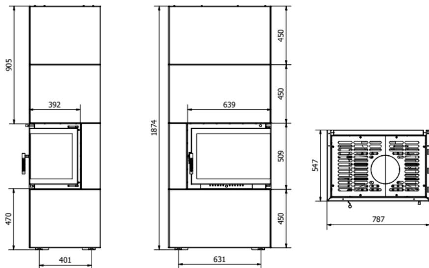
Figure 1: A dimensioned installation drawing of the SIMPLE BOX in BSP version
