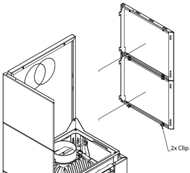
**Step 16.** Prepare the double front panel, top panel as shown in the diagram below.
