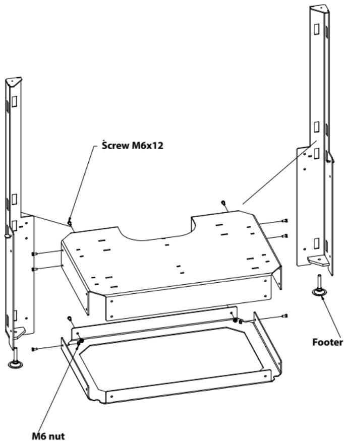
**Step 2:** Following the steps of step 1, screw the front legs of the superstructure in accordance with the diagram below.
