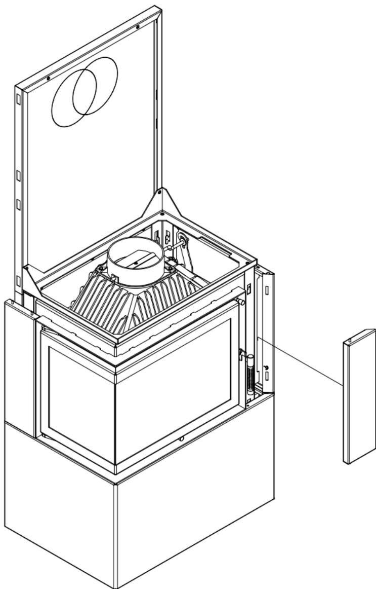
**Step 14:** Prepare the two double side panels for installation as shown in the diagram below. Both panels will be in mirror image - the number of hooks at the bottom of both panels differs for the BSL and BSP versions of the unit (see drawings below). The upper fastening screws should also be screwed only partially (a few threaded coils), as was the case in the lower panels, so as to leave room for mounting the upper frame, the supporting structure of the installation.
