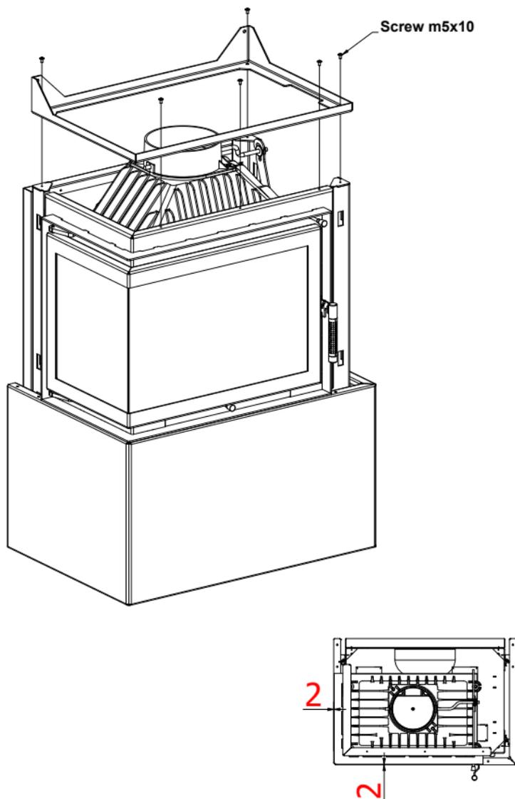
**Step 9:** Install the top panel as shown in the diagram below by screwing it to the superstructure.
