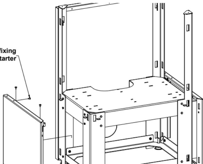
**Step 6** As shown in the diagram below, mount the front-bottom panel by inserting it using the hooks in the notches in the side-bottom panels
