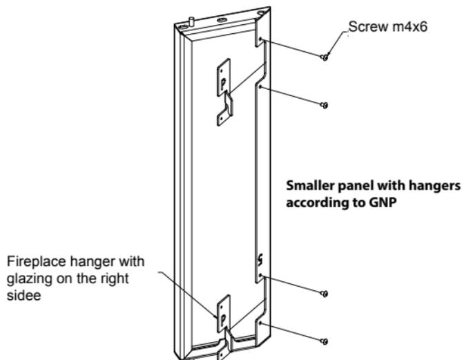
**Step 13:** Install the smaller front panel by sliding it into the notches in the side panel and substructure as shown in the diagram below.
