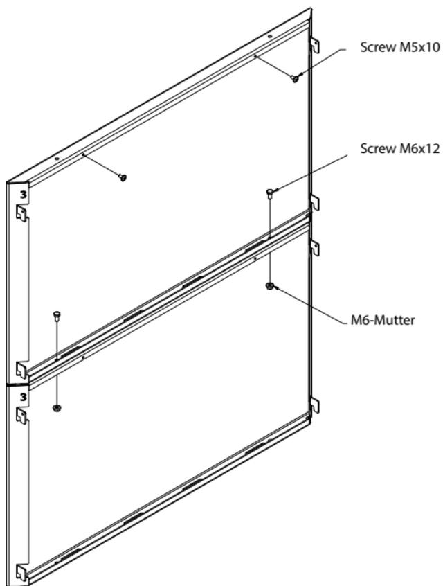
**Step 17:** Install the front cover plate as shown in the following figure by inserting it into the recesses in the side panels using the hooks.
