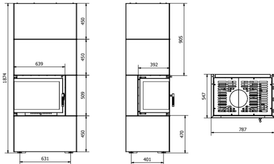
Figure 2: A dimensioned installation drawing of the SIMPLE BOX in BSL version
