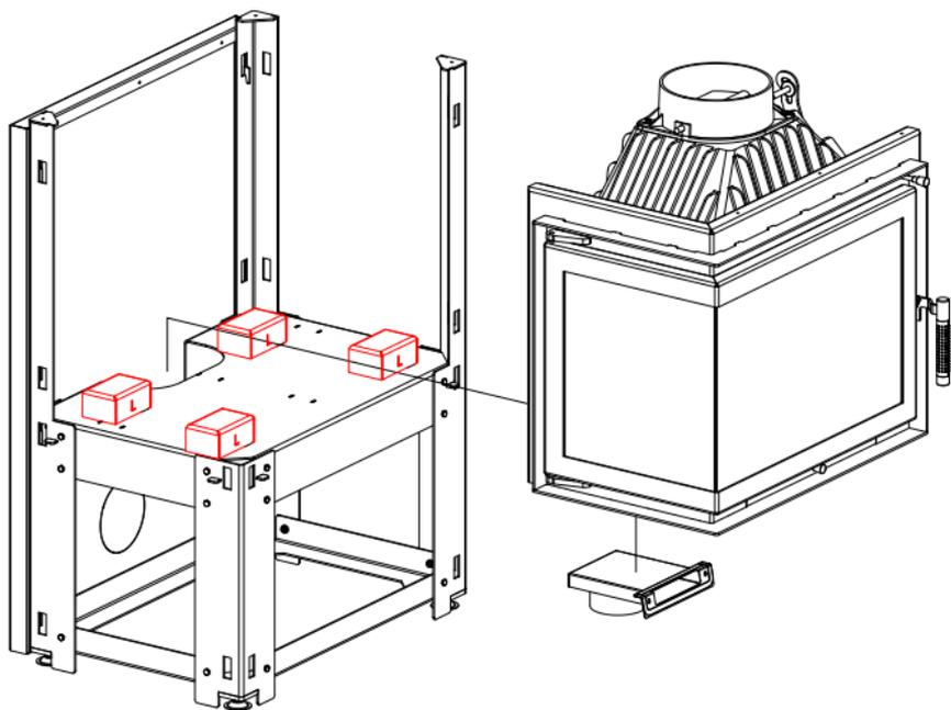
**Step 4:** In the next step, install the side panel according to the diagram below, inserting it using the hooks in the notches in the substructure. Use the M5 screws in the diagram below to level the side panels in the first case. The M5 bolt used to fix the hook should only be partially screwed in, leaving room for the hook as shown in the diagram in steps 10 and 11.
