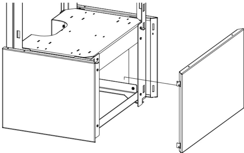
**Step 7:** If you have not installed the inlet, this means that the unit is not yet installed on the substructure, so in the next step place the unit on the substructure as shown in the diagram below.
