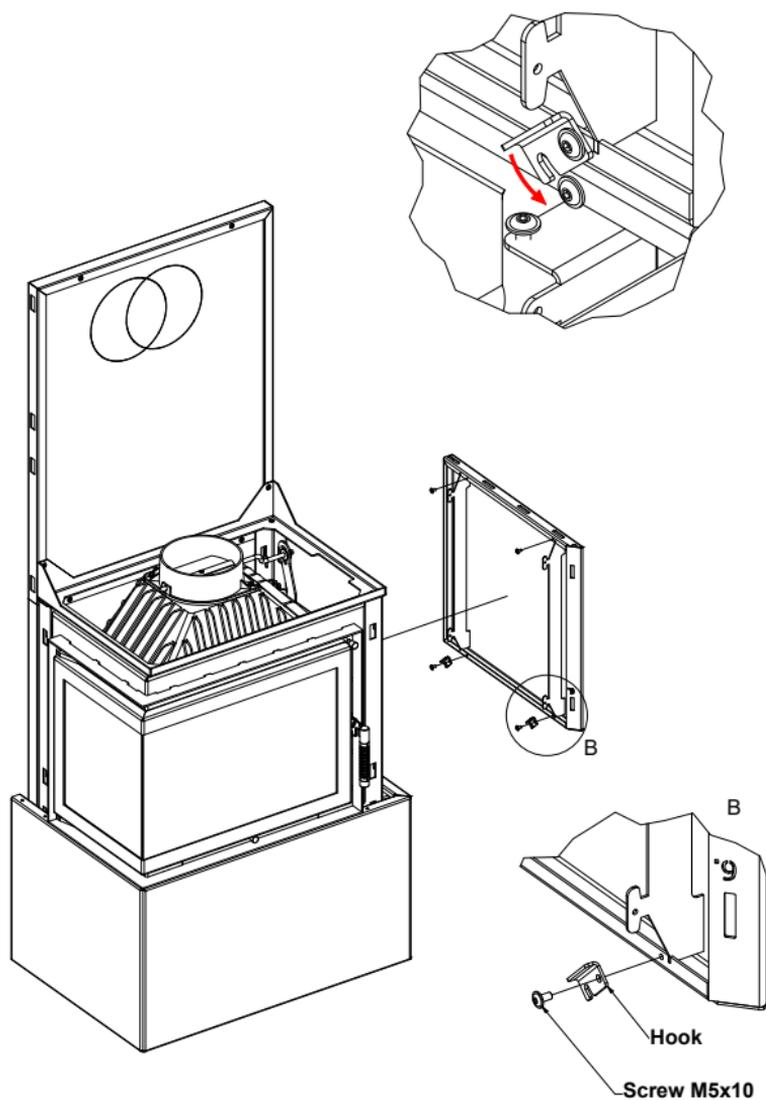
**Step 11.** Similar to step 10, install the smaller side panel on the opposite side of the superstructure.
