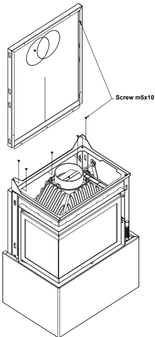
**Step 10:** Insert the side panel by inserting it into the notches in the substructure, using the hooks that must be fastened after inserting it according to the diagram below. Before installation, screw the hooks as shown in the diagram below and screw the hook screws to the top of the side panel by only partially screwing it in (a few coils of thread) to leave room for the hook of the top panel.
