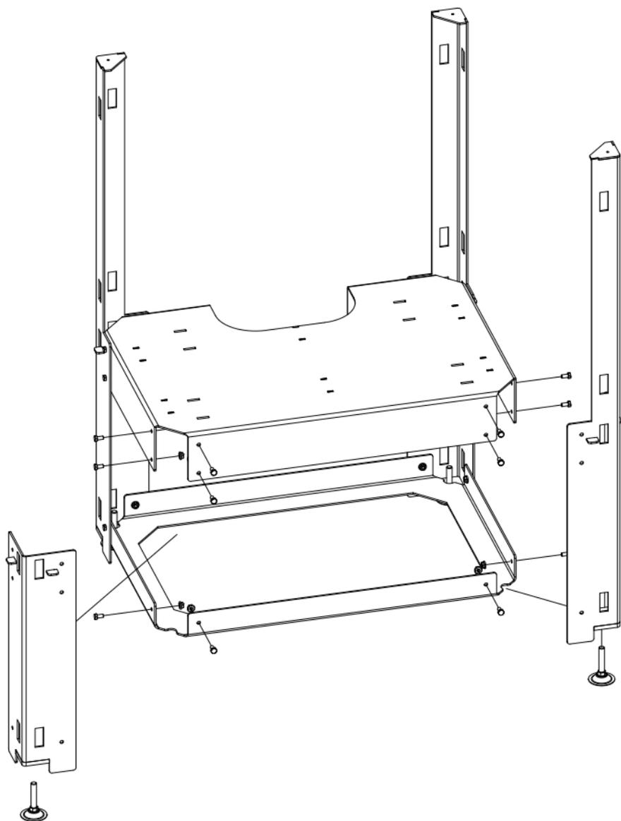
**Step 3:** Install the back panel, as shown in the diagram below, using the hooks on the panel and inserting it into the notches in the substructure frame.
