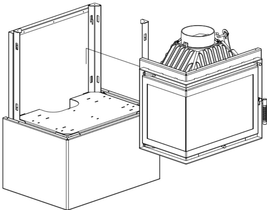
**Step 8:** Mount the frame of the upper part of the superstructure as shown in the diagram below. The diagram also shows that the side and front panels should extend 2 mm beyond the flange of the fireplace frame.
