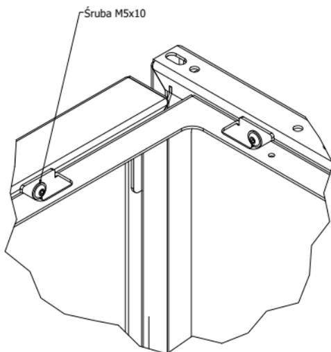
**Step 19:** Install the top cover plate by screwing it to the previously installed frame of the substructure, as shown in the diagram below.
